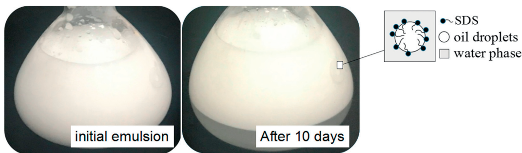
Fig. 2. Stability of ethanol/water/2-ethyl-1-hexanol/SDS system.
